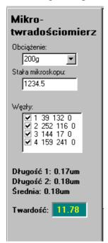
Before the measurements are made, weight which was used for the test is to be chosen (in grams) and constant values for a microscope and measurement system are to be provided (in pixels/millimeter).
