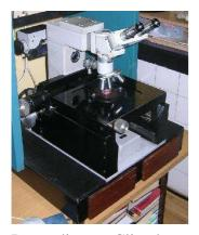
Upgrade of a microscope is possible thanks to the use of photo converter (as in the case of high definition video camera or photo camera converter). We use only Canon photo cameras in our project. Joining optical track is possible with prism or eye-piece.
