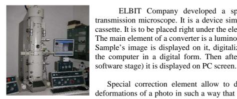
ELBIT Company developed a special converter for transmission microscope. It is a device similar in size to a film cassette. It is to be placed right under the electron gun. The main element of a converter is a luminophore plate. Sample's image is displayed on it, digitalized and next sent to the computer in a digital form. Then after pre-processing (in
