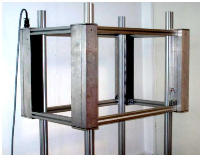
Photooptic gates are used to measure the velocity of flying bullets. There are many horizontal photoelectric barriers built in the frame of the gate. A bullet flying through the target causes disruption of one or more lines, which can be detected by frame's acceptance photoelements.
